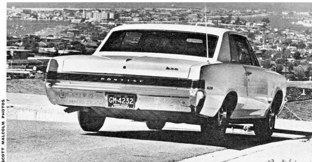
GTO BOASTS the cleanest lines of the A-body GM series, has stop, tail and turning lights integrated into rear trim. Exhaust splitters poke out behind wheels.
