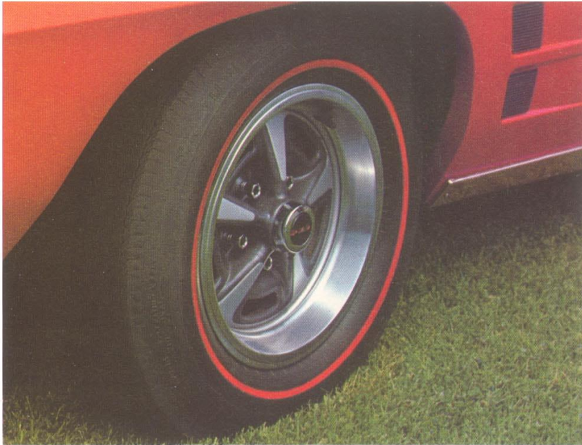
Rally II Wheels (Code 454—UPC N98). Available on all models. New and larger, 15" diameter for Catalina, Executive and Bonneville. 14" diameter on Firebird, Tempest, Custom S, LeMans, LeMans Safari, GTO and Grand Prix. Stamped steel gives appearance of magnesium. Chrome plated wheel nuts. (Conventional spare wheel provided with space saver tire.) (F)
