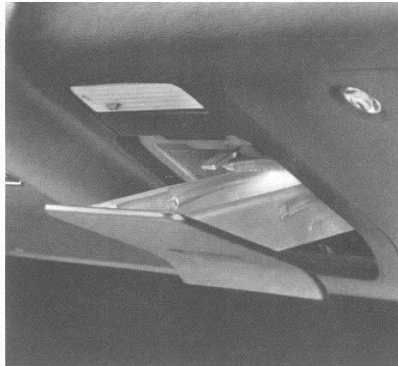
Ashtray Lamp (Code 662—UPC U28). Available for Tempest and Custom S models only—included in Lamp Group (Code 322). Standard on all other models, all series. Lights automatically when headlights are on. (F,D)
