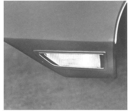
Cornering Lamps (Code 651—UPC T87). Available for all models except Firebird. Part of Lamp Group (Code 322). Lights up blind spots when turning. Goes on when headlights are on and turn signal is activated. Mounted on forward side of front fender. (F)
