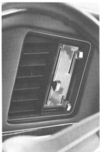
Automatic Temperature Control Air Conditioning Controls for Grand Prix.
