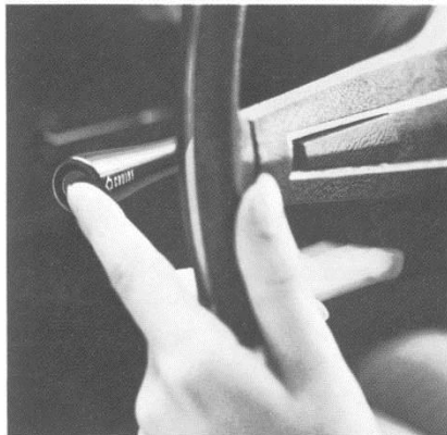
Cruise Control (Code 441—UPC K30). Select your speed, and it will stay there until you disengage by lightly touching the brake pedal (available on all models with V-8 engines and automatic transmissions only). (F,D)
