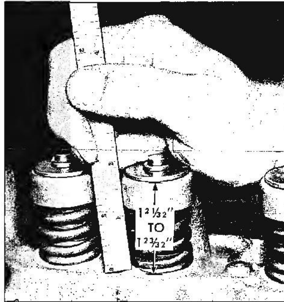
Fig. 6-34 Checking Valve Spring Installed Height
