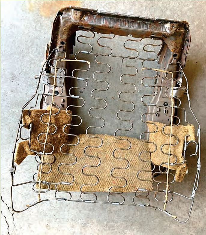
Figure 3. This is what your seat bottom looks like with no upholstery or upper padding. The remaining padding can stay on if it is still serviceable like here. Note the paper coated listing wire that is used to attach hog rings so the side bolsters have definition from the center seating area. More on that later.
