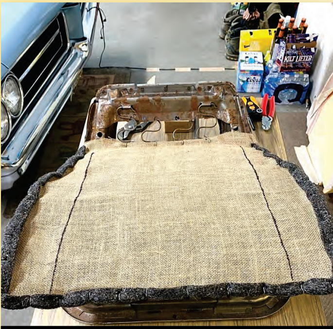
Figure 6. You can use a black Sharpie to trace over the factory paper-coated listing wire in the seat springs as a guide to make sure everything lines up. This is important when you install the foam cushion and fasten the paper-coated listing wires in the pockets hanging off of the bottom of the upholstery to the listing wire in the seat springs. If you want, you can install a new listing wire on top of the burlap and over the original.
