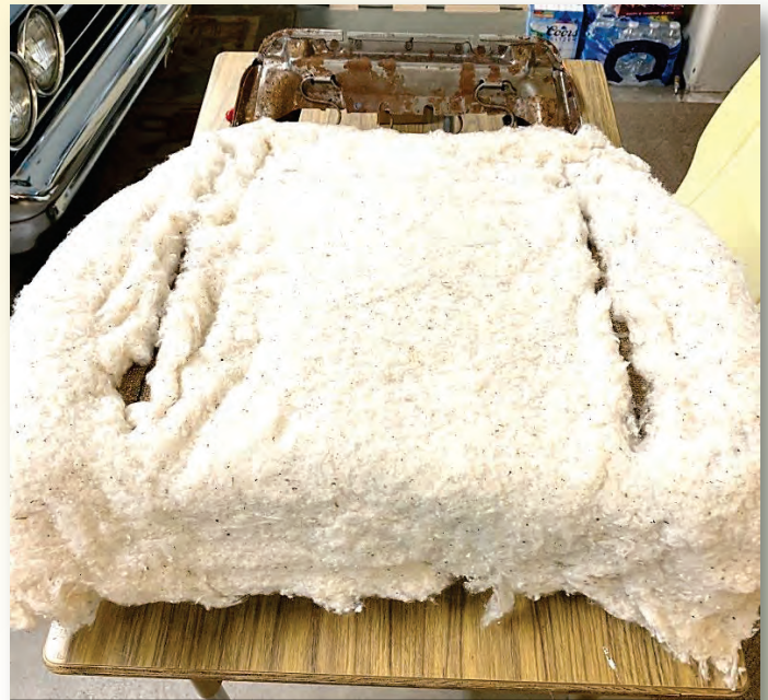
Figure 7. Install a single layer of cotton padding over the burlap and pull apart slits over the listing wires as shown.
