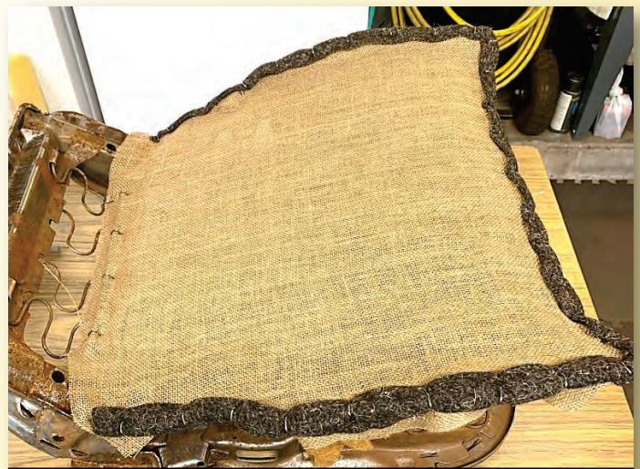
Figure 5. Two inch felt is installed around the edge to prevent the springs from sawing into your new seat foam or upholstery. Again, spacing of hog rings is about ever 2-3 inches.
