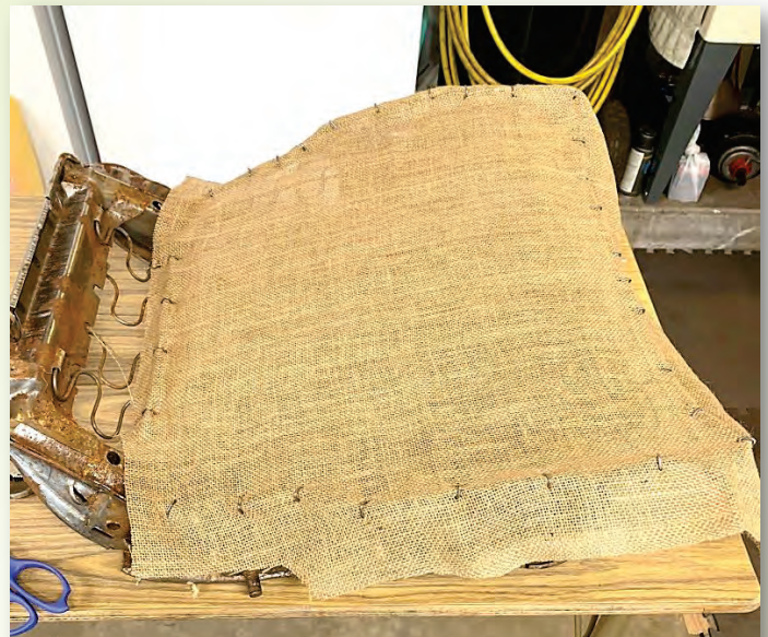
Figure 4. Putting a single layer of burlap on the seat springs is the first step in reupholstering the bucket seat bottom from my 1964 GTO. Note the spacing of hog rings around the perimeter.
