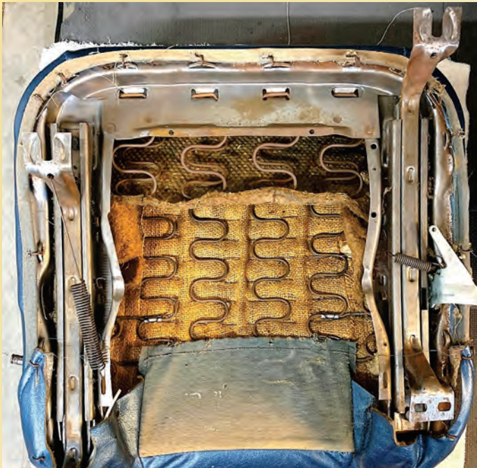
Figure 1. Notice the hog rings all around the skirt bottom of the seat and the gray panel pulling the rear portion of the upholstery tight.
