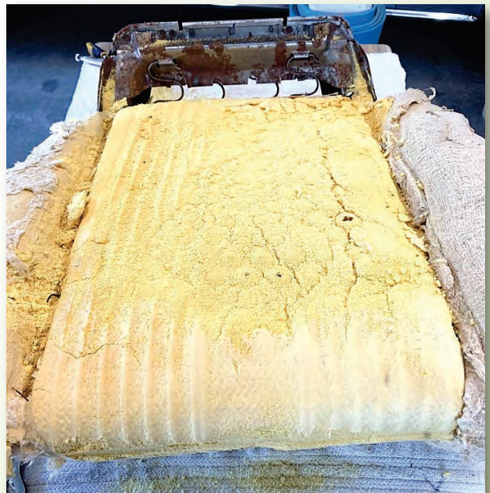
Figure 2. Decaying foam is obvious in this photo. You can see the grooves in the seat where the listing wires formerly resided along the inside of the side bolsters.
