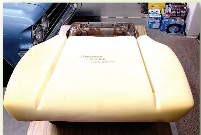
Figure 8. The seat cushion goes over the cotton and the slits you cut in it should align with everything underneath (e.g., slits in cotton, black line, listing wires in seat springs).
