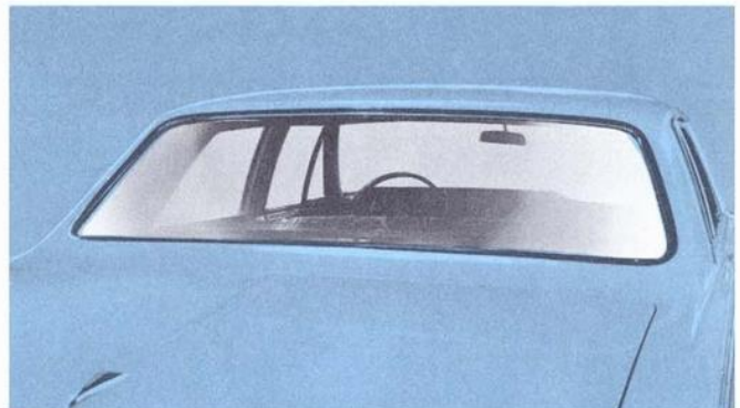
Rear Window De-Fogger (Code 541) . . . blower under rear package shelf directs air through grille to rear window for clearer view. (See illustration on Page 5.) (D)
