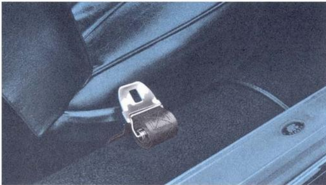
Seat Belts and Seat Belt Retractor (Code 624) . . . outboard belts retract to compact roll when not in use, extend to needed length when in service. Belts meet highest safety standards. Choice of harmonizing colors. (D)
