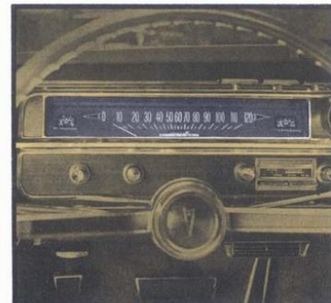
Custom Gauge Cluster (Code 504) . . . gives more complete engine information, with oil pressure and water temperature gauges. On Catalinas, electric clock is mandatory. Not available with Electro-Cruise or Safeguard Speedometer. (F)
