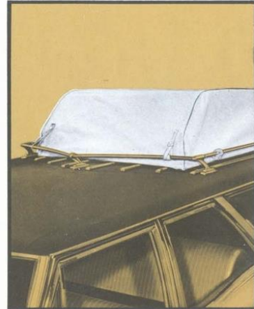
Luggage Carrier Cover. Water and dust-resistant fabric protects luggage. Side opening can be locked. Cover folds flat when not in use. Easily attached to Safari Chrome Luggage Carrier (Code 571). (D)
