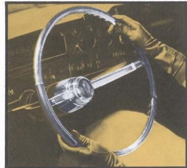
"Wonder-Touch" Power Steering (Code 501) . . . drive, turn, park with ease. One to two pounds effort sufficient for steering, yet retains feel of control. (F,D)
