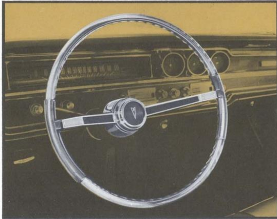
Deluxe Steering Wheel (Code 461) . . . all new, redesigned and restyled, featuring a horn activator bar recessed into each of the two wheel spokes. Standard on Star Chief, Bonneville and Grand Prix; optional on Catalina. (F,D)
