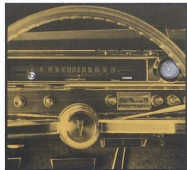
Safeguard Speedometer & Fuel Warning Lamp (Code 634) . Warns of excess speed and low fuel. Control knob lets you select desired speed limit. Buzzer and light signal you when car exceeds this speed. (F)
