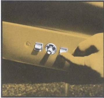
Power 6-Way Seat (Code 561) . . . redesigned for added stability in unlimited seat positions for greater comfort and safer driving. Available full-width front seat only. (F)
