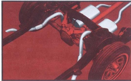
Dual Exhausts (Code 511) . . . available on the 326 V-8 engine. (Standard on the 326 HO V-8 and on GTO Option.) Cuts down exhaust back-pressure, adds to engine efficiency. (F)
