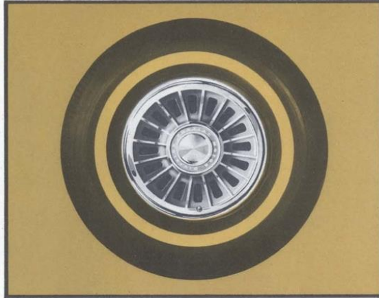
Deluxe Wheel Discs (Code 462) . . . chrome-flashed stainless steel. Redesigned with deep center section and all-new appearance of a stronger, bolder wheel. Standard on Star Chief, Bonneville and Grand Prix; optional on Catalina. (F,D)
