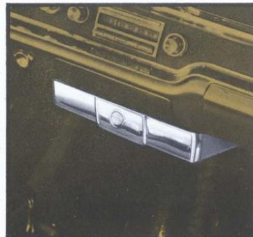
Tissue Dispenser . . . holds a regular-size Kleenex box. Mounts under instrument panel. Swings out for use, swings back when not needed. (D)
