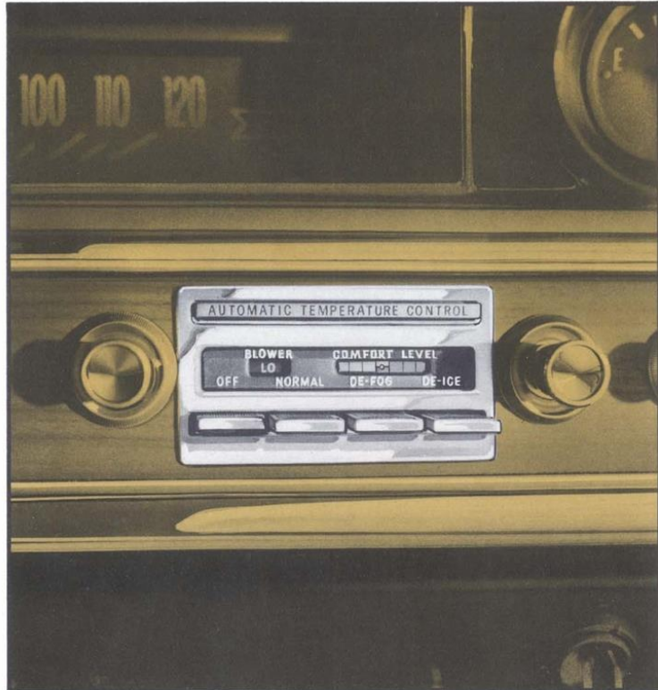
Automatic Temperature Control Air Conditioning (Code 581). Dial on instrument panel lets you preset desired comfort level. Automatic control maintains comfort regardless of weather. At any temperature over 35°F., removes excess moisture from air limiting window fogging. (F)
