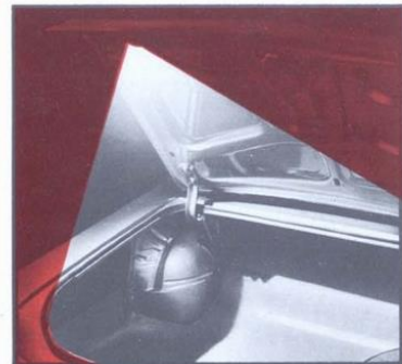
Luggage Lamp (Code 481) . . . automatically turns on when trunk lid is lifted. Reflecting shade directs light to every area of trunk . . . frees hands for loading, unloading luggage. (F,D)
