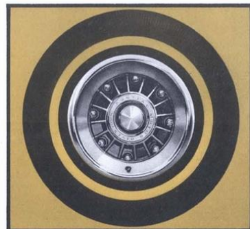
Aluminum Wheels and Brake Drums (Code 691) . . . distinctive one-piece aluminum wheel hub and brake drum bonded to cast iron braking surface . . . virtually immune to brake fade. (F)
