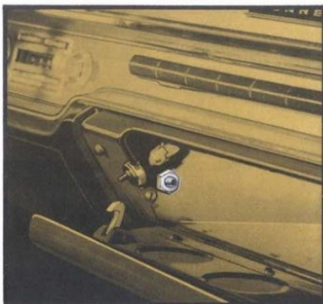
Rear Deck Lid Release (Code 451) . Lets you open trunk from driver's seat without removing key from ignition. Push-button control located inside glove box. Trunk may also be opened by key. All models except Safari. (F,D)
