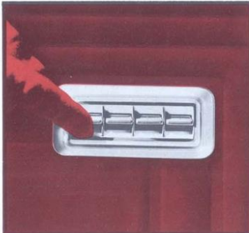
Power Window Lifts (Code 551) . . . for automatic control of all vertically opened windows from single control on door trim at driver's position. Individual controls at each window. (F)
