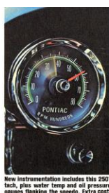
New instrumentation includes this 250° tach, plus water temp and oil pressure gauges. Pinstriping the speeds. Extra cost.
