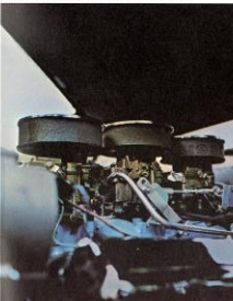
Two extra-cost engines. Both Tri-Power. Horsepower—376 and 376. Cubic inches—421. Carburetor—3-2BBL. With mechanical linkage on stick shift jobs. Dual exhausts.
