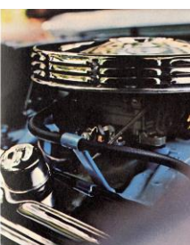
The standard engine. Horsepower—338. Cubic inches—421. Carburetor—4BBL. Dual exhausts. Channeled low-restriction air cleaner, rocker covers, oil filter cap.
