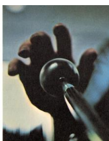
A fully-synchronized, heavy-duty 3-speed with short-throw Hurst floor shifter comes standard on the 2+2.
