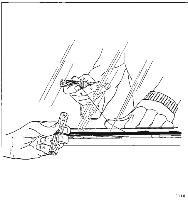
Fig. 2E17—Adhesive Caulked Window Removal
