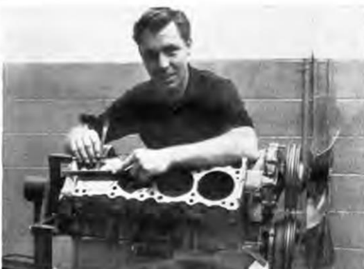
ABOVE —Sid Warren carefully measures the block deck clearance to the minimum .0015 during blue-printing of the engine. This attention to detail is where you pick up that additional horsepower needed to win.
