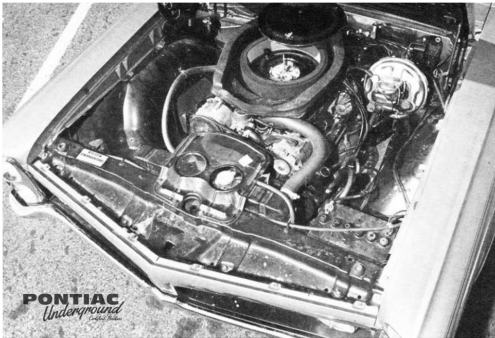
FOAM BOOT seals rammed air into plenum chamber. Air cleaner element can be removed to eliminate restriction for competitive dragstrip work.
