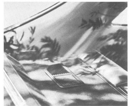
Rear-window Defogger (Code 404). A blower under the package shelf channels air through a directional grille out the rear window. Helps give you a clear view when inside windows have tendency to fog up. Available on all models except station wagons and convertibles other than Firebirds. (F, D)
