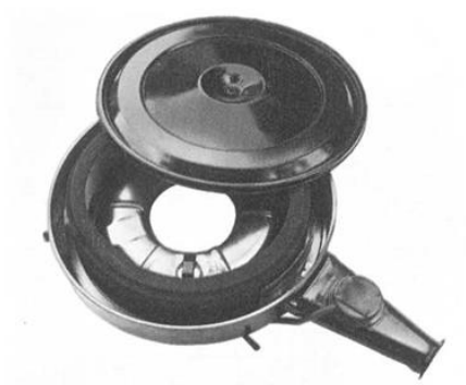
Dual Stage, Heavy-duty Air Cleaner (Code 731). Dual-filter design consists of wetted paper in filter, surrounded by polyglycol wetted polyurethane foam outer filter. Fine filtration, extended surface. Available all models except those equipped with 428 H.O. engines. (F, D)
