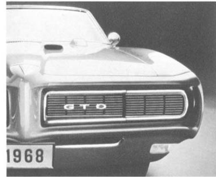
Concealed Headlamps—GTO (Code 414). Available only on GTO models. Provides a distinctively clean appearance to the front end. Sections of the grille swing down and out of the way when headlamps are in use. Headlamp switch automatically controls position of headlamp doors. (F)
