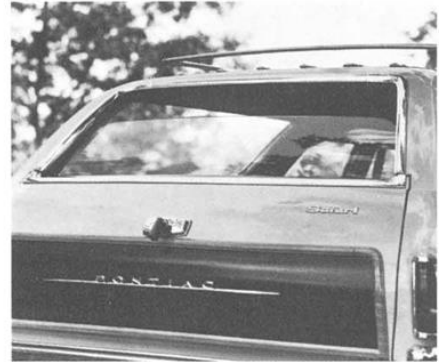
Power-operated Tailgate Window (Code 542). Conveniently located switch raises or lowers tailgate window at touch of finger or twist of key in tailgate lock. Available for Catalina and Executive 2-seat, Tempest Custom and Tempest Safari Station Wagons only. (Standard on all 3-seat station wagons) (F)
