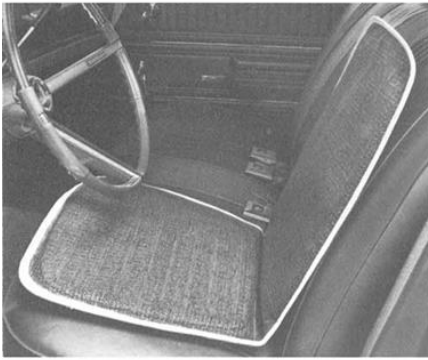
Ventilated Cushions. Helps make driving more comfortable, especially in hot, sticky weather. Special, coil-spring construction allows air to circulate between passenger and seat. (D)
