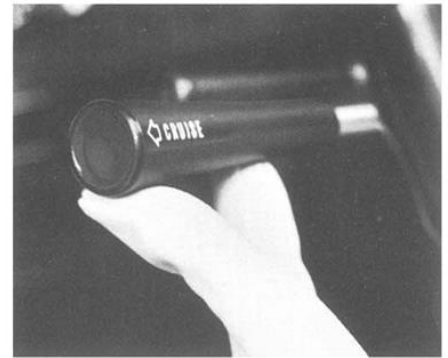
Cruise Control (Code 441). Maintain a pre-selected car speed automatically. Disengages with slight touch of the foot on the brake pedal. Available on all models with V-8 engines and automatic transmissions only. (F, D)
