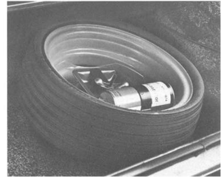
Space-Saver Spare Tire (Code 702). Adds up to 3 cubic feet of usable luggage capacity. Easily inflated with handy pressure can and affords approximately 2,000 miles of spare tire driving. Available on all models. Standard on Firebird series. (F). New Space-Saver Tire inflators for replacement are available at your dealer. (D)
