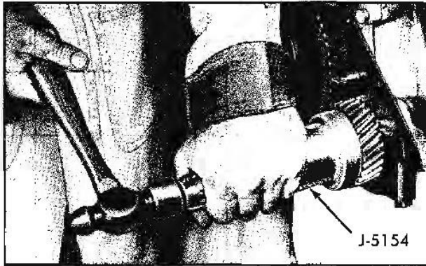
Fig. 6-76 Installing Crankshaft Timing Gear
