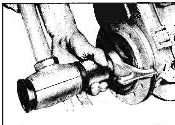
Fig. 6-42 Installing Harmonic Balancer
