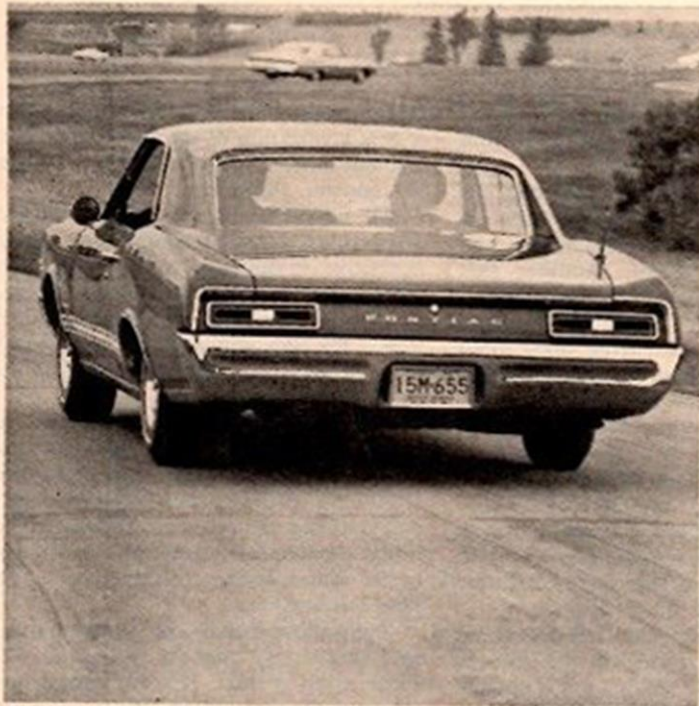
Backup lights emphasize 3-part tail lamp assemblies used on all Tempests except GTO. This is Le Mans Sprint with ohc-6.
