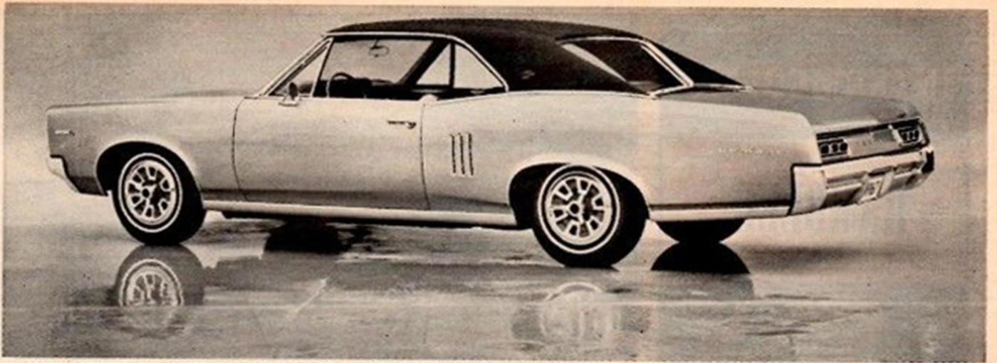
LE MANS HARDTOP HAS RECESSED REAR WINDOW. STANDARD 165 HP COMES FROM BELT-DRIVEN, SINGLE-OVERHEAD-CAM, 6-CYLINDER ENGINE.
