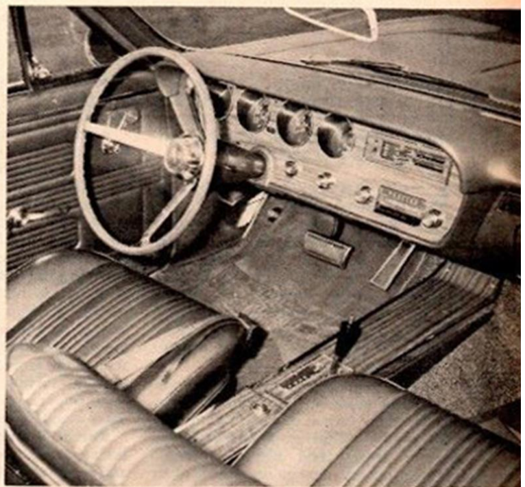
GTO with automatic has console-mounted selector. 1st and 2nd may be manually engaged by pressing button on shift knob.
